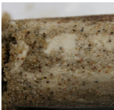
(b) gravels intrusion in the sand layer
